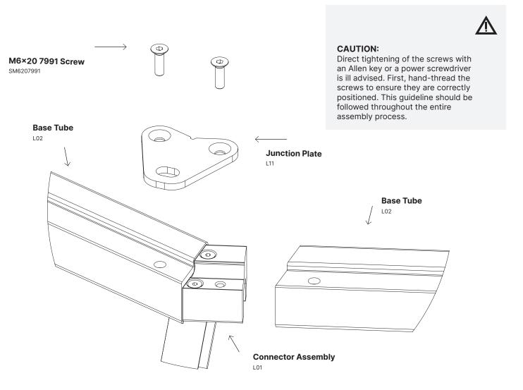
Insert the connector assembly into the base tube, followed by another base tube on the opposite side. Secure these components using the junction plate and M6×20 7991 screws.
